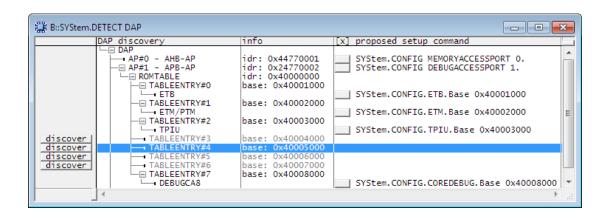
However, TRACE32 does not rely on the ROM table. If the chip is supported by TRACE32, then it is enough to select the right CPU using the command
