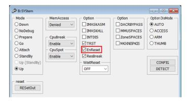
Please also check if the reset line of the debugger is properly connected to the chip reset (like the reset button).
