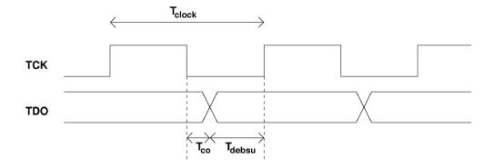
For the debugger this means the target chip will generate data on the **TDO** signal with a setup time of **Tdebsu** = **Tclock/2** - **Tco** . The hold time of the data will be **Tco** + **Tclock/2**.
