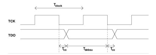
So in this case the target generates a setup time for the debugger of Tdebsu = Tclock - Tco.
