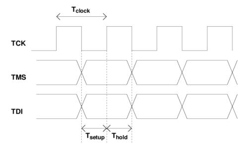
The target chip should sample the TMS and TDI signal on the rising edge of TCK.
