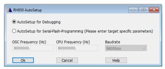
Set the mode to "AutoSetup for Debugging" then press OK.
