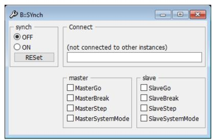
Otherwise, you can get a hardware-based synchronization if the chip supports BDGREQ and DBGACK signals. In this case, you can connect both debug modules over PODBUS and use the commands **TrBus.Out Break ON** and **TrBus.Set Break ON** for each PowerView instance. This type of synchronization is however not supported for synchronous start (**Go**).
