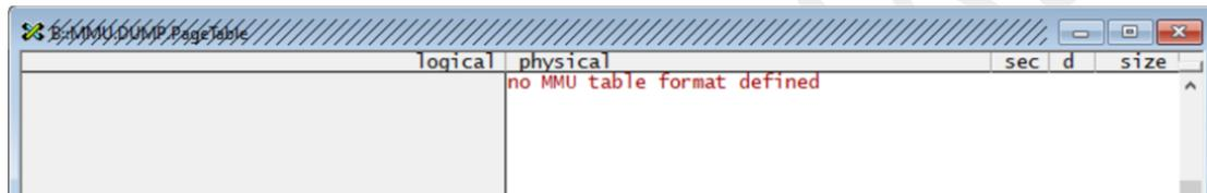
To resolve this, use the `MMU.View` command to inspect the current values of the MMU-related registers and verify that they are correctly initialized.
