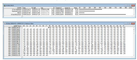
If TRACE32 is configured to expect a different pattern than the one actually used by the operating system, it will incorrectly report 100% stack usage in **TASK.STacK**.
