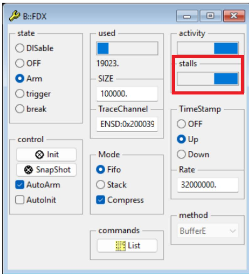
At certain times, the volume of generated trace information exceeds the capacity of the trace channel. Consequently, the FDX target code must wait until the channel becomes available. This behavior intentionally introduces stalls and affects the run-time performance of the target application in order to avoid trace data loss. The likelihood of stalls strongly depends on both the amount of trace data being exported and the characteristics of the target processor.
