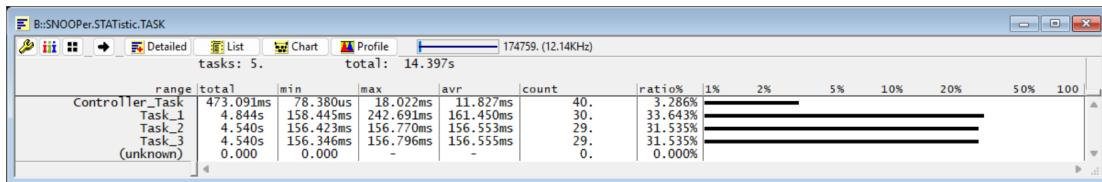
While the total function run-times show only a relatively small deviation, the accuracy is noticeably lower. This reduced precision is particularly evident in the longer average and maximum values.
