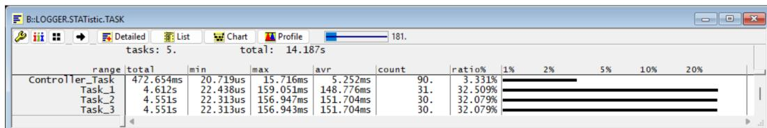
By comparing the two results, we observe only minor deviations in the total, average, and maximum task run-times between LOGGER and off-chip trace. A more pronounced deviation appears in the minimum run-time values, as the logging overhead tends to mask very short execution times. The table below summarizes the differences for `Controller_Task` as an example.
