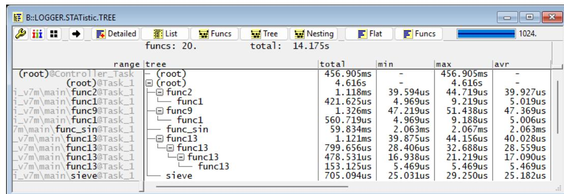
The next screenshot shows the runtime results of the non-instrumented code, obtained through off-chip trace
