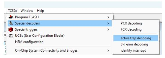
If the core is halted *inside* the Trap Service Routine (not at the trap vector itself), the AREA window may display "No exception detected." This is expected because the core has already moved past the trap vector.
