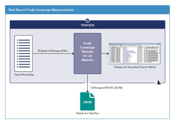
After concluding the test run, the outcomes for all source code metrics, stored within TRACE32's internal code coverage system, can be exported to a JSON file. Supported source code metrics include statement, decision and condition coverage, MC/DC, as well as call and function coverage. Export is restricted to functions with loaded symbols.
